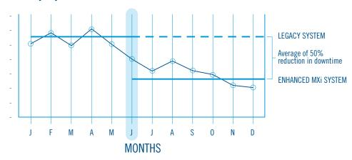
The enhanced MXi system was installed in June and helped G&D improve uptime by 50 percent in six months.
