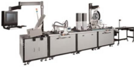
The Datacard CPST MJ7500™ card personalization system provides much faster output than conventional thermal printing, with comparable image quality.
