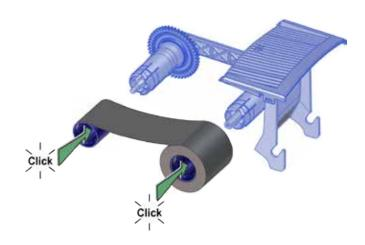
c. Load the cleaning sleeve onto the ribbon cartridge.
