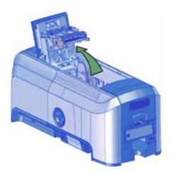
c. If the printer has the optional multi-hopper, unlock the printer and open the printer supplies access door and the multi-hopper cover.
